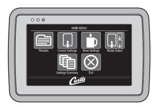
3 The MAIN MENU screen contains a series of submenu icons. The icons vary based on the model selected under the Model Select sub-menu. For the brewer to operate properly, the model selected must match the model series on the brewer model number label affixed to the outside of the machine.
