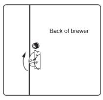
1 The brewer should be ON. Confirm this at the rear toggle switch. "Ready to brew" should be on the display. If the brewer is connected to an inter-lock grinder, the grinder should be on. When inter-lock connection is made, grind coffee at this time.
