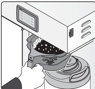
4 Slide the filled brew basket into the brew rails under the control panel. Slide it all the way back until it stops.
