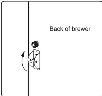
1 The brewer should be ON. Confirm this at the rear toggle switch. “Ready to brew” should be on the display. If the brewer is connected to an inter-lock grinder, the grinder should be on. When inter-lock connection is made, grind coffee at this time.
