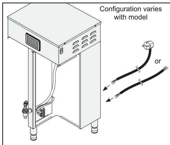
**Connecting the Brewer Wiring (Units That Come from the Factory Without a Power Cord Attached)**
