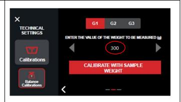
4) Place a preset weight on the group scale and wait 15 seconds before pressing "CALIBRATE WITH SAMPLE WEIGHT".
