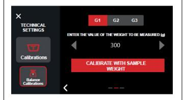
6) Calibration is complete and the weight may be removed from the group scale.
