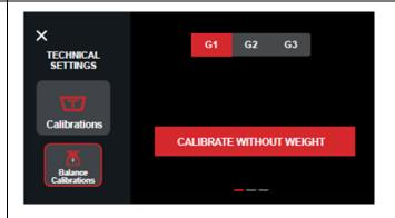
3) Set the chosen weight for calibration (a weight of 300g is suggested, max 500g).
