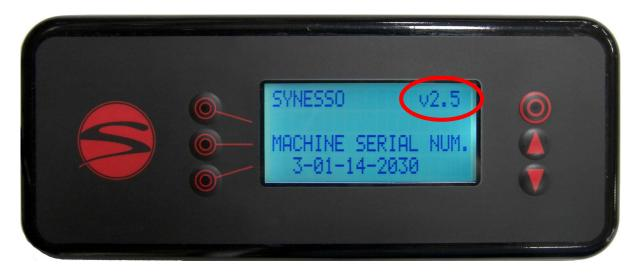
The start-up screen appears momentarily when the machine power is cycled on. The firmware can be viewed in the upper right corner of the screen, in this case v2.5.
