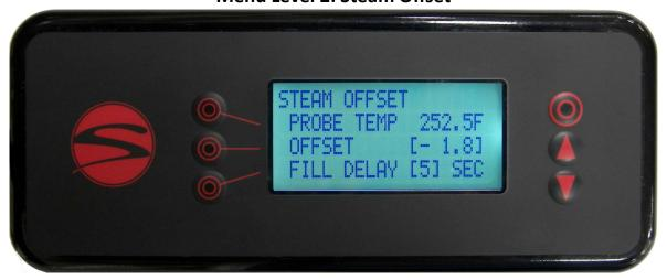
Line 2 indicates the measured steam temperature at the steam tank temperature probe.
