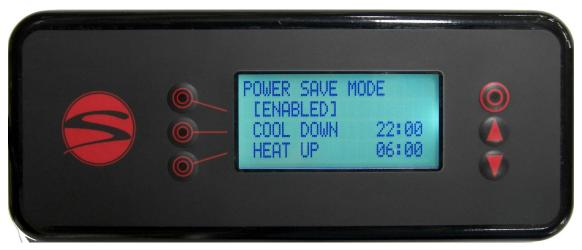
Line 2 of the Power Save Mode in this example is indicating the timers are [ENABLED], making adjustments to lines 3 and 4 available. If line 2 reads [DISABLED], no further settings will be available on this screen.
