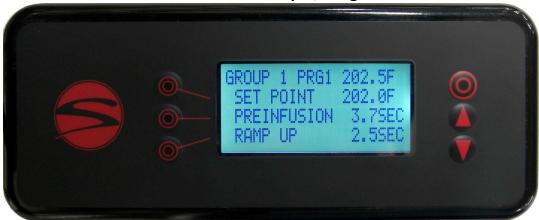
Line 1 of the first brew group control screen indicates the current temperature of the brew tank as measured by its probe. Once this temperature reaches the set point, it will continuously cycle up and down by small increments as the electronics balance the temperature. This line also indicates the active program (PRG1 in this case). Changing the active program will update the settings on the lines below.
