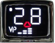
Steam Tank, Low Water **Level or Low Flow Error**
