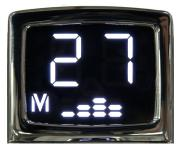
2 Bars: Bypass Pressure Ramp Down
