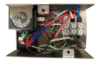
To connect the power cord: Insert the color coded pump cable into the opening of the matching bypass box and attach the wires to the terminal as shown in the picture to the left: green wires stacked on the ground bolt, white matches across to white/red on terminal block, black matches across to black/blue on terminal block, and the male bullet connector on the black wire connects to the female bullet connector on the red wire.
