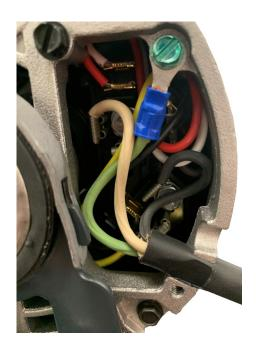
To connect the power cord: Secure the ring terminal on the green grounding wire to the frame of the motor using the green screw. Insert the spade connector of the white wire to the upper terminal. Insert the spade connector of the black wire to the lower terminal. Blank spade connectors are installed in factory on the terminals that should not be used in the motor. Never connect the white and black wires to the same brass terminal plate.
