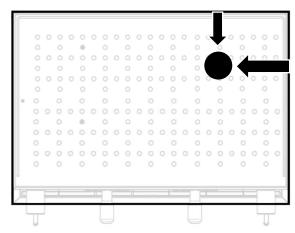
2.5" hole in counter recommended for passage of electrical cord & water/drain lines.
