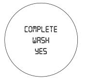
Select by pressing buttons (A) or (C), then press button (B) to confirm. The following screen will be displayed:
