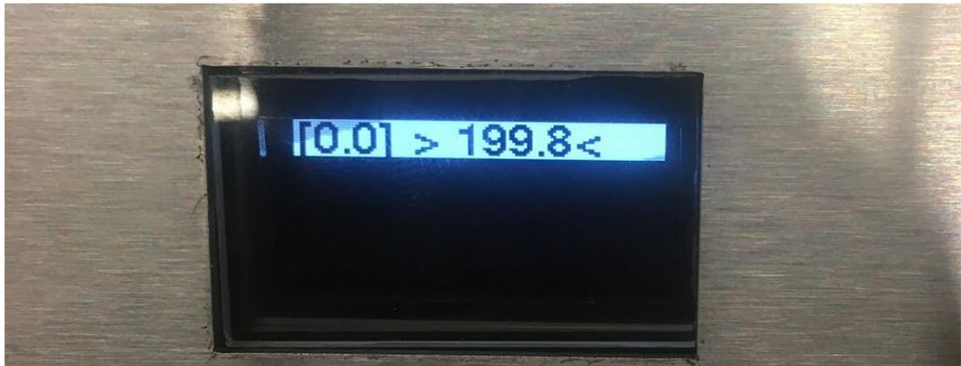
When changing the offset use the Pre-Infusion and Brew actuators to increase or decrease the offset until the displayed temperature matches the measured temperature.
