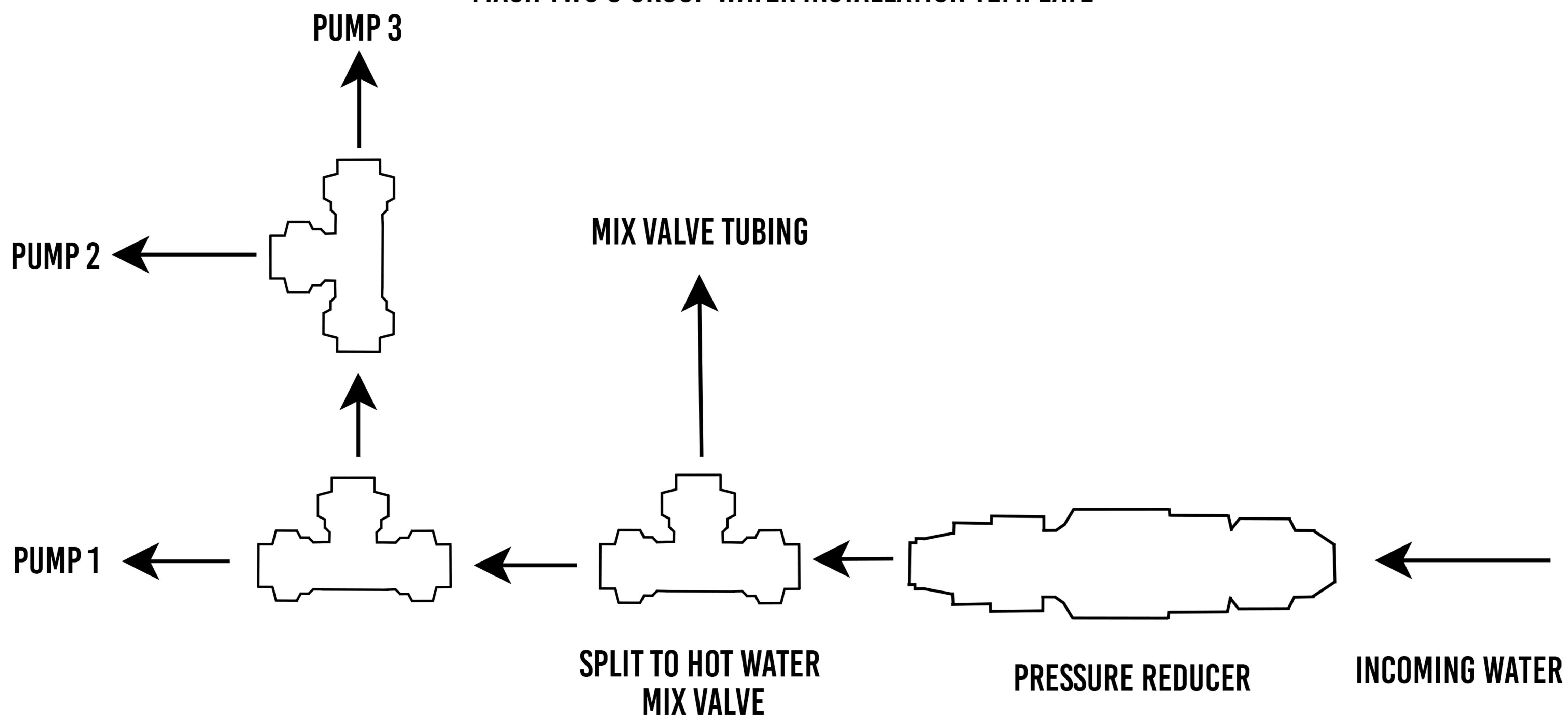
THE PRESSURE REDUCER PLACEMENT IS VERY IMPORTANT, WITHOUT IT PRE-INFUSION AND THE HOT WATER TAP WILL NOT FUNCTION AS INTENDED
