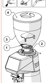
Using a soft-bristled brush (clean and sanitised) and a vacuum cleaner, remove the coffee beans and coffee powder residue from the grinding chamber (Part. 1).
