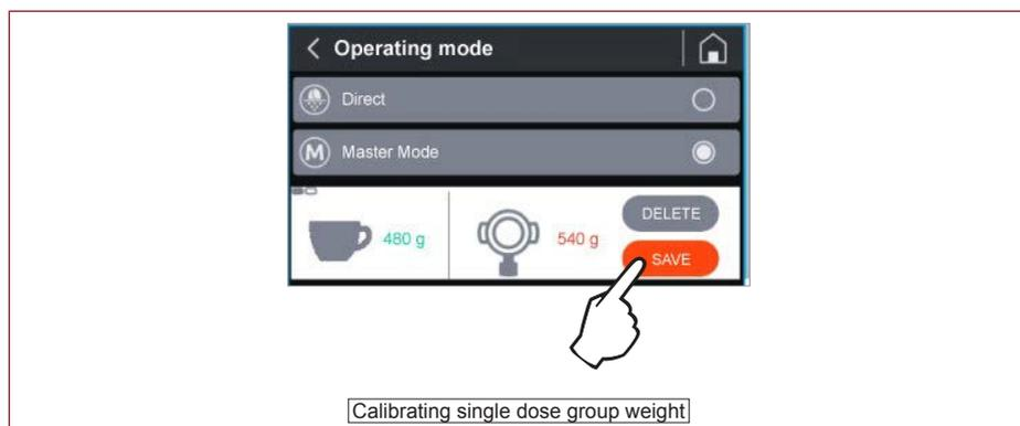
On resting the portafilter on the holder, the machine automatically detects the weight of the portafilter and dispenses the set quantity of coffee.
