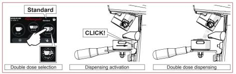
Fig. 12 - Double dose dispensing in 'Standard' mode.
