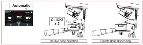
Fig. 14 - Double dose dispensing in 'Automatic' mode.
