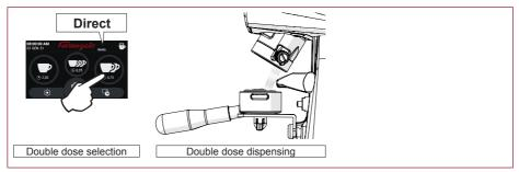
Fig. 13 - Double dose dispensing in 'Direct' mode.
