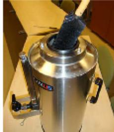
First, remove the black funnel assembly. Then, using a cleaning brush, scrub out the liner thoroughly, loosening coffee oils into the water.
