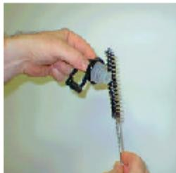
Unscrew the faucet and remove the rubber seat cup. Clean using the sight tube brush.
