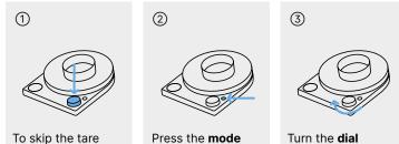
step, start with your button to toggle empty container on between the three the weigh pan, and modes, selecting Weight.
