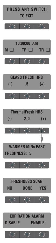
If a carafe is placed on a particular warmer, a "box" will appear next to it's indicator. If the box is filled (solid) it's not expired yet. If the box is empty, the time is expired. See example: MAIN = expired; Top Front = not expired; Top Rear = expired. Press right hidden button to advance to next function.
