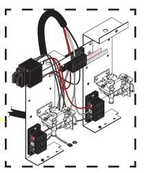
**Note:** Power cord must be connected to <u>center terminal</u> <u>block</u> on all Twins unless otherwise noted.
