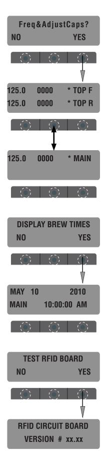
This allows you to monitor the frequency of the warmer(s) sensing coils.
