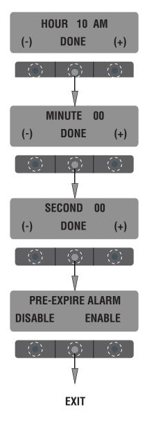
Press "+" to scroll hour forward, or "-" to scroll hour back.
