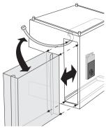
Remove the tank from the side of the machine. Clean the inside with water.
