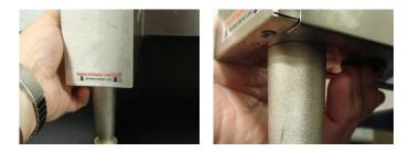
2. Turn off Main Breaker IF THE BREWER IS HARD WIRED LOCK OUT BREAKER & SKIP TO STEP 4
